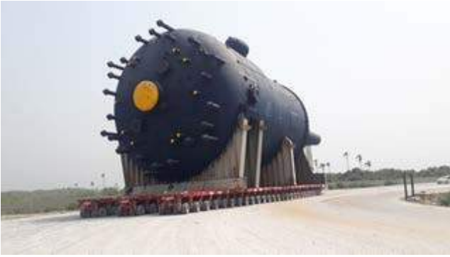
Fig. 8: Reactor Transportation in Single Piece
