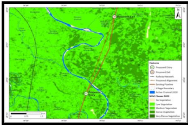
Figure-10 Spatial distribution of the river between 1985 and 2025 concerning the existing GAIL pipeline network. The analysis highlights progressive shifts in the river's course driven by variations in flow dynamics, rainfall intensity, and seasonal hydrological regimes
