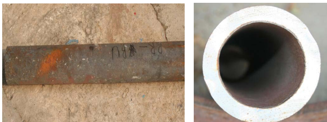
Fig. 1: As received photograph of tube Samples (external and internal surface)
