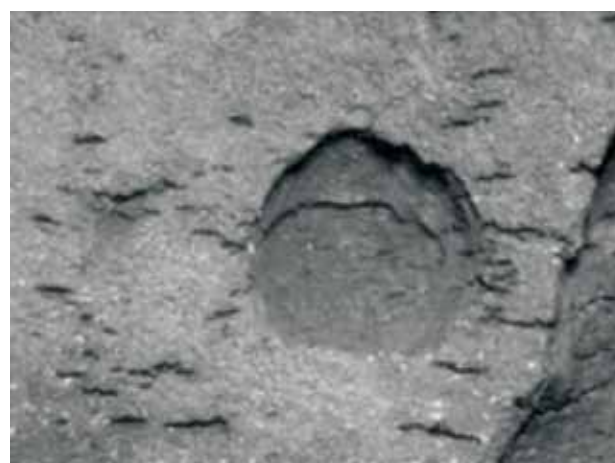
Figure 5: Low Magnification Examination 10 x of production tubing internal showing progressive pits
