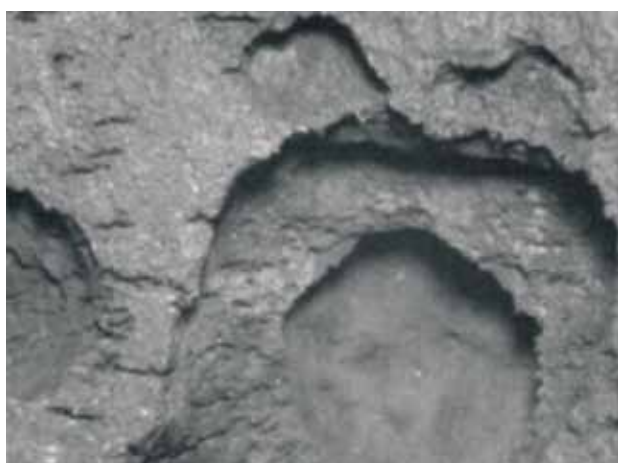
Figure 5: Low Magnification Examination 10 x of production tubing internal showing progressive pits
