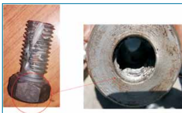
Figure 7: Erosion corrosion failure of choke at a gas well
