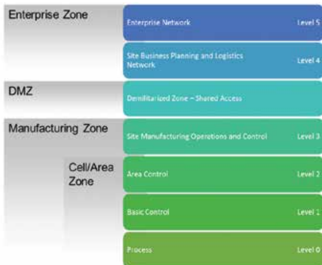
Figure 3 Purdue Enterprise Reference Architecture model on the left and IIoT Reference Model on the right
