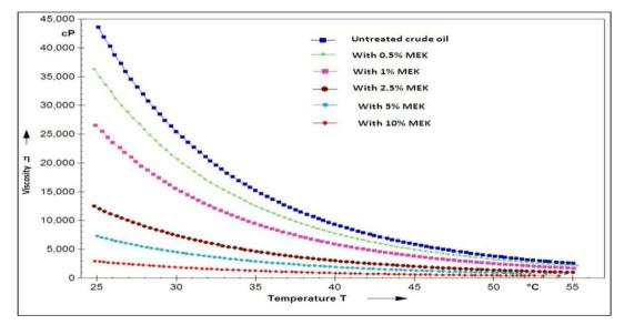
3.7 Effect of blend of MEK and MTO with EGMBE at lower concentrations on the viscosity of crude oil:
